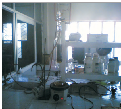
Fig-1- Soxhlet apparatus for extraction
