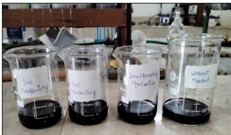
Figure-5 Four equal parts of 200ml solution for pre, post and simultaneous mordanting with natural mordant and without mordant
